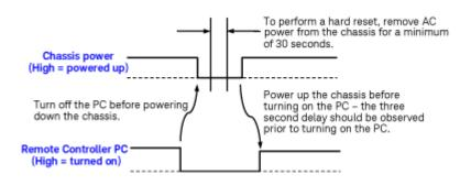
In essence, a chassis hard reset is a system restart that includes unplugging the chassis from AC power after the chassis is powered down.
