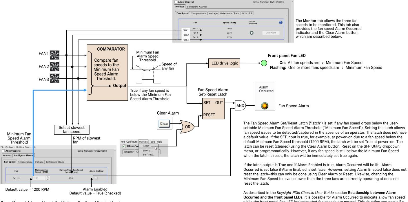
The **Configure Alarms** tab is used to set the Minimum Fan Speed threshold and enable/disable the Fan Speed Alarm. The Minimum Fan Speed can be set from 1 to 10,000 RPM either by entering the value directly or by using the up/down arrow buttons. As an aid in setting the Minimum Fan Speed, the current value of the slowest fan is displayed.
