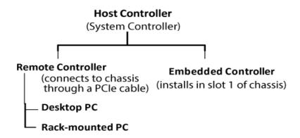
The host controller can either be a remote controller or an embedded controller. A remote controller is a Windows-based PC, and can be a desktop PC or a rack mounted PC. The remote controller interfaces to the chassis through a PCIe cable.
