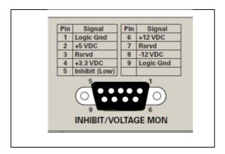
Each voltage rail contains a current limiting resistor to prevent accidentally shorting the supplies during measurements.
