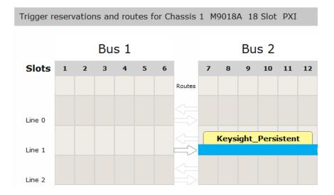
To create a route from Bus 1 to Bus 2, the PXI-9 specifications require only the destination segment (Bus) to have a reservation. This is why only one of the arrows shows a solid line. If you had reserved both lines, both Bus 1 and Bus 2 segments could be the destination of the route and both arrows would have solid outlines indicating that a route in that direction is allowed.
