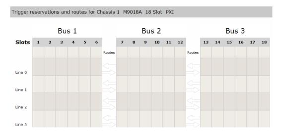
3. To reserve trigger line1, place the cursor onto Line 1 area inside the Bus 2 column and then click.
