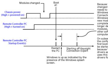
Because the chassis configuration has changed since the last boot, sufficient time needs to be allowed between when Windows is up and when Keysight Connection Expert is started to ensure that Windows is able to assign drivers to the new modules that it finds. This is usually completed within one minute, but can take longer depending on the number of new modules, the speed of your computer, and other software being executed as the computer boots up.
