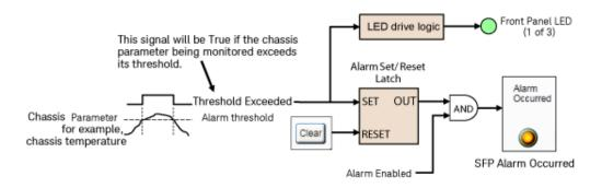
In this example, the Threshold Exceeded signal will be True if the chassis parameter being monitored exceeds its threshold. For example, if a temperature sensor reports a temperature greater than the temperature threshold. A True value of Threshold Exceeded causes the following:
