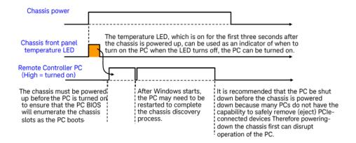
The PC should be shut down before the chassis is powered down. This will prevent the chassis, as it is being powered down, from disrupting operation of the PC.
