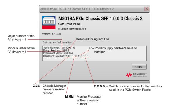
The **Hardware Revision** contains four numbers representing four chassis components the chassis firmware revision is the first number listed. Of the four components whose revision numbers are being reported, only the chassis firmware is customer upgradeable. Information on upgrading chassis firmware is provided below.
