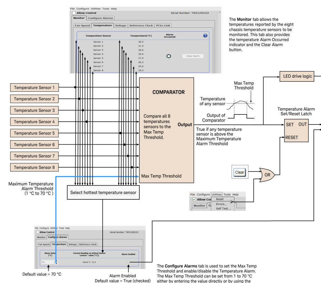
up/down arrow buttons. To aid in setting the Max Temp Threshold, the current value of the hottest temperature
