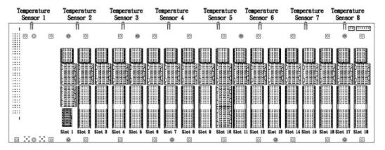
By knowing the location of the temperature sensors relative to the chassis slots, you can determine which modules are potentially contributing to excessive temperatures. To address this, you can take steps such as redistributing modules in the chassis or installing air inlet modules adjacent to high power modules to provide additional ventilation.
