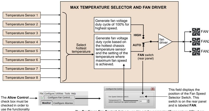
The **Configure Fan Control** dialog is used to set the parameter "Temperature (°C) where maximum fan speed achieved" – this parameter will be referred to by its IVI.NET driver name, MaxRPMTemperature. At SFP startup, the SFP reads the chassis value of MaxRPMTemperature and inserts that value here. The chassis default value is 50 °C.
